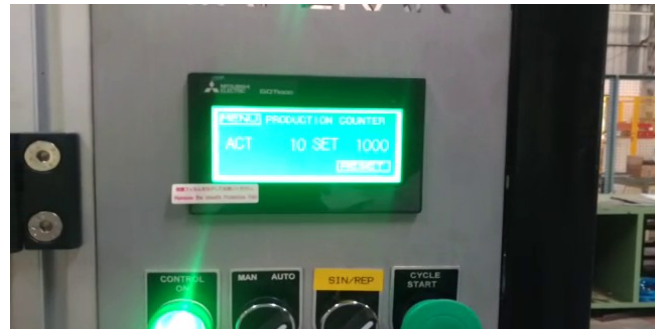
PLC With HMI for Braid Cutting Length Setting
